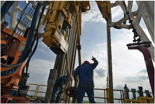
A floor hand signals to the driller to pull the pipe from the mouse hole on Orion Drilling Co.'s Perseus drilling rig near Encinal in Webb County, Texas, U.S., on Monday, March 26, 2012. The Perseus is drilling for oil and gas in the Eagle Ford Shale, a sedimentary rock formation underlying an area of South and East Texas. Photographer: Eddie Seal/Bloomberg
